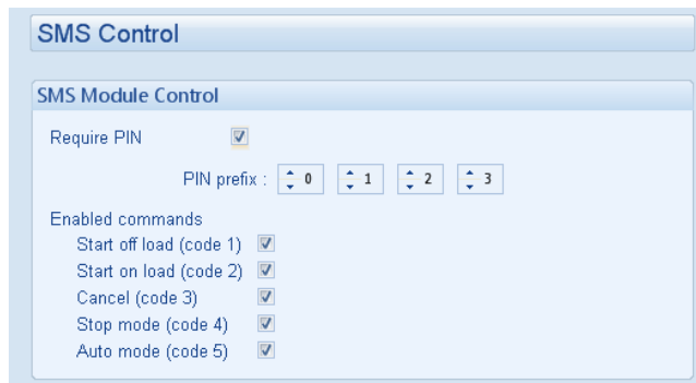
Example screen shot of SMS Control setup in the DSE Configuration Suite
